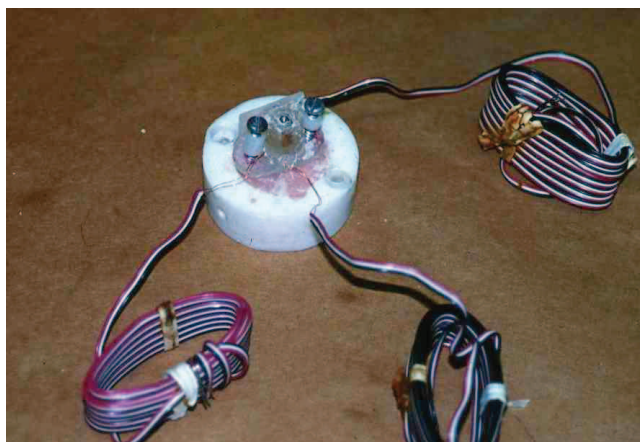
FIGURE 3. A completed specimen with the strain gages attached. The implant is in the center of the sample. The leads from the strain gages attached to the acrylic extend outward from the sample.
